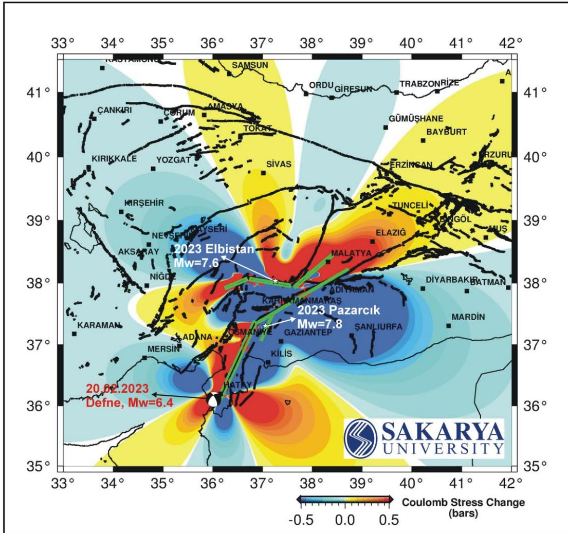
**Figure 6.** Coulomb stress changes due to the 2023 Pazarcık and Elbistan earthquakes calculated along the fault plane of the February 20, 2023 Defne aftershock.
